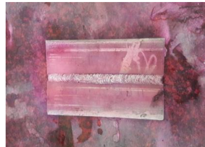
Fig. applying penetrant
