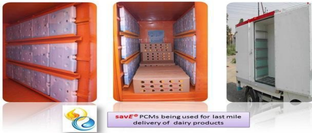
Fig. 2.10: Cooling Of Dairy Product (www.pcmproducts.com)
