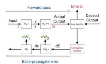
Fig -2: Backpropagation Network
