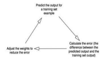
Fig -1: Backpropagation Network Flow
