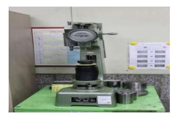
The Brinell method applies a predetermined test load (F) to a carbide ball of fixed diameter (D) which is held for a predetermined time period and then removed. The resulting impression is measured with a specially designed Brinell microscope or optical
