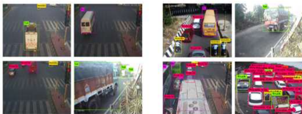
Sample images with object detection bounding box and class label outputs
