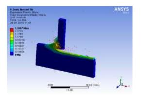
Fig 12: Equivalent plastic strain at 70m/s & DOC 2mm
