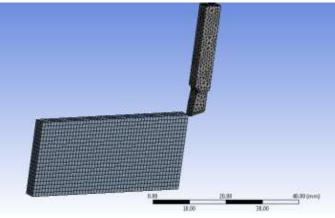
Fig 6: Meshing for work piece and steel4340 tool
