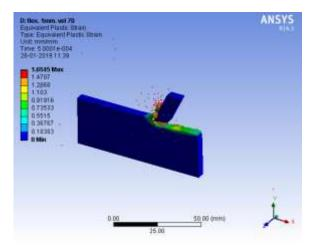
Fig 7: Equivalent plastic strain at 70m/s & DOC 1mm
