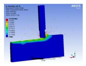
Fig 11: Equivalent plastic strain at 70m/s & DOC 1mm
