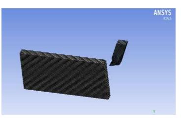
Fig 5: Meshing for work piece and tungsten tool
