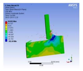
Fig 14: shear stress at 70m/s & DOC 2mm
