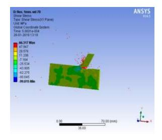
Fig 9: shear stress at 70m/s & DOC 1mm
