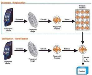
Fig.3. Working of Fingerprint
