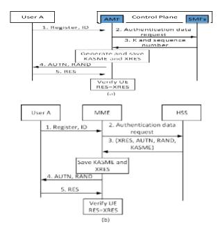
FIG 7- Verification dependent on various security design.
