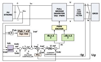
Fig -4: Control of single phase inverter using PLL
