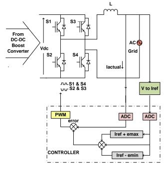
**Fig – 6:** Hysteresis current control for grid connected inverter
