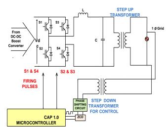
Fig -5: Grid connected inverter using ZCD circuit
