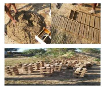
Fig -2: Preparation of specimen
