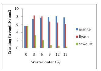
Chart -1: Crushing strength Vs waste content
