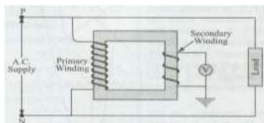
Fig.3.7 Circuit of Potential Transformer
