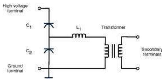
**Fig.3.7(c)Simplified Circuit Diagram Of A CVT**
