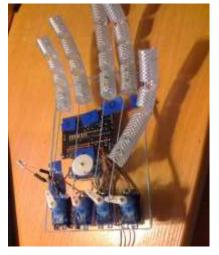
Fig 5: Mechanical arm using servos
