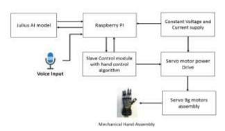
Fig. 2 : Block Diagram of HandSpeak System
