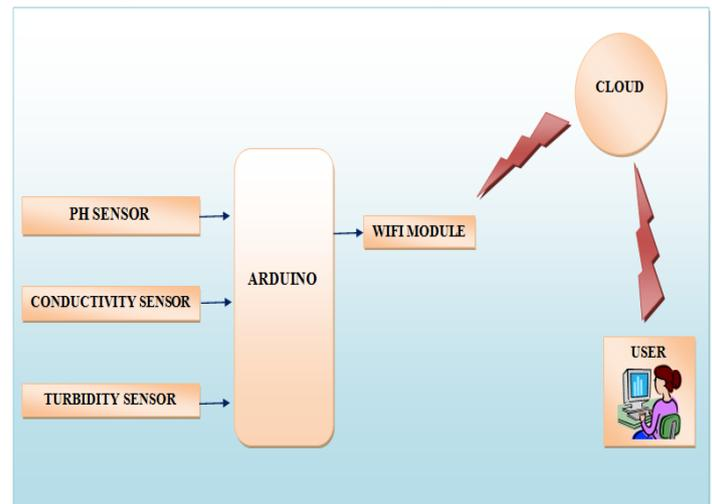
of water goodness by using IoT has been proposed. Internet of things together with the Sensor water meters for the effectiveness, govern the quality of water. Here we are executing, system for monitoring the water goodness through different sensors-turbidity, pH, temperature, conductivity. The controller accesses the information which is monitored by the use of sensors. The accessed data is controlled by the usage of Arduino controller. By using an IoT, the information
