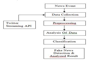
Fig -1: Block Diagram
