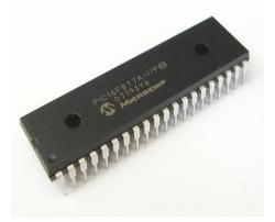
Fig. 2.2: PIC16F877A Microcontroller
