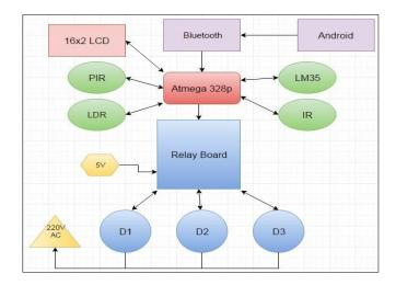
Fig. 1: Block Diagram of Home Automation
