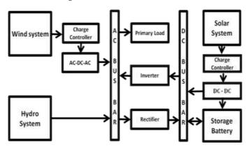
Figure1. Structure of hybrid wind-PV-hydro power generation system
