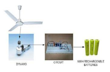
Fig. 3.1: Charging NIMH Batteries using Dynamo
