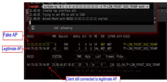
Figure 9: A fake AP powered on with airbase-ng tool in BackTrack5
