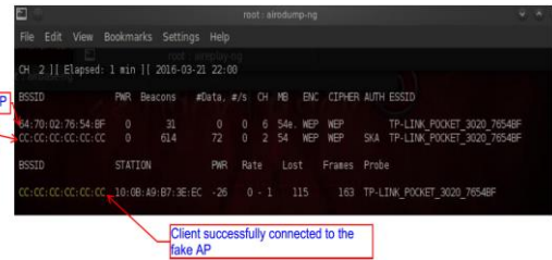
Figure 11: The legitimate client successfully connecting to the fake AP
