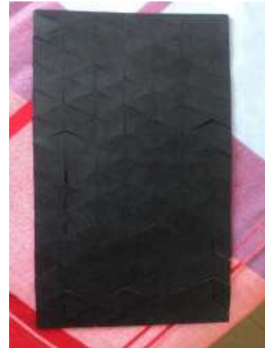
Figure 5 Auxetic Structure made from Rubber Sheet
