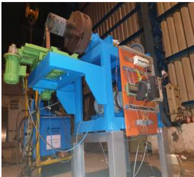
Fig -7: Side view of manufactured weld overlay machine
