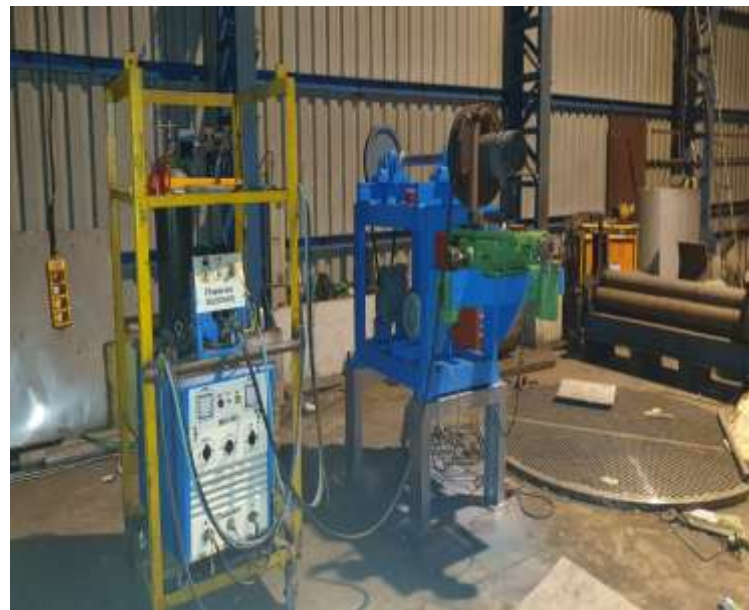
Fig -9: Final Assembly of Weld Overlay automation with welding apparatus
