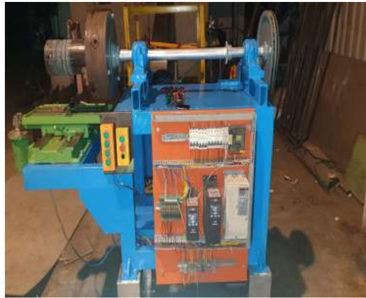
Fig -8 Front view of manufactured weld overlay machine
