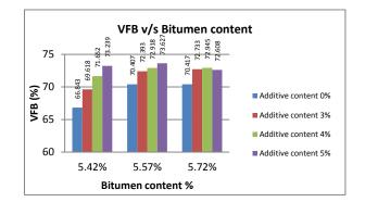
NOTE: With increase in additive content it was observed that voids filed with bitumen increases for binder content 5.42% and 5.57 % but in case of binder content 5.72% voids filled with bitumen first increases upto 4% additive content but further addition of additive content decreases the value of VFB.
