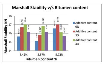
**NOTE:** With increase in additive content the load value of warm mix increases and also greater than the control mix. The load value increases upto addition of 4% additive. Beyond this the load value decreases. Maximum load value is achieved at 4% additive content for all binder contents.
