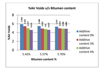
**NOTE:** Air voids in percentage decreases with increase in additive content for all the binder contents and also lowers than the control mix.
