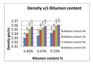
**NOTE:** It was observed that when the additive is added in the control mix its density starts increasing with increase in additive content for all the binder contents.
