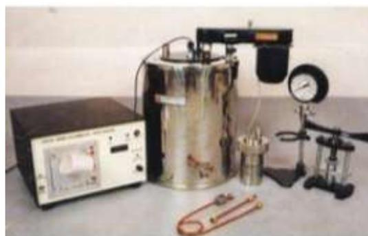
Fig -5. Setup for evaluating Calorific value
