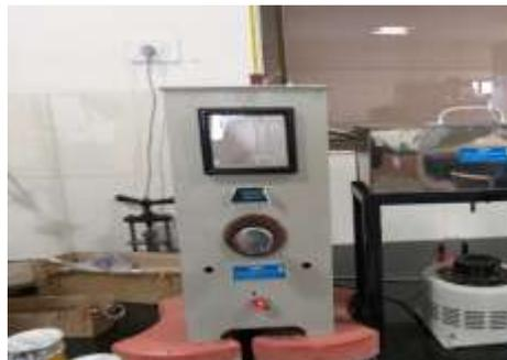
Fig -4 ASTM -86 Distillator (manual)
