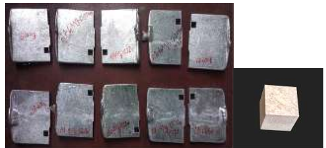
Fig. 4.9 Samples for EDAX and microstructure analysis
