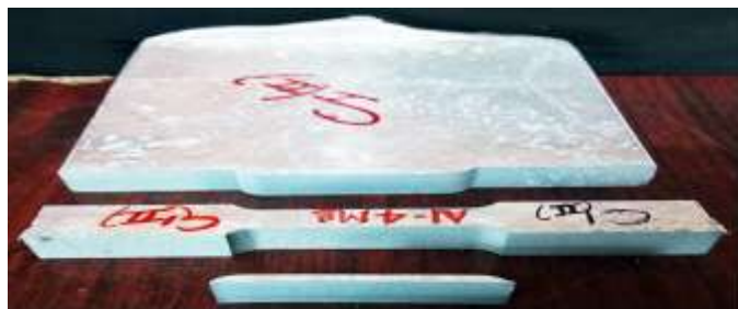
Fig. 4.7 Procedure of tensile specimen preparation
