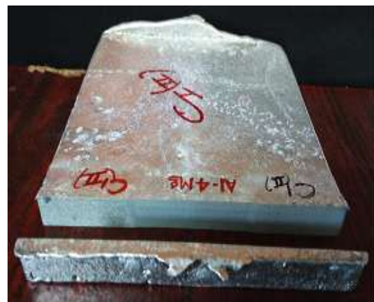
Fig. 4.5 Initial cutting by EDM
