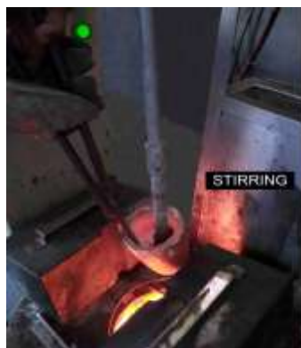
Fig. 4.2 Stirring molten metal in mould cavity
