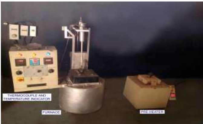
Fig. 4.1 Induction furnace & Preheater
