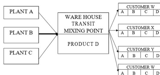
Fig. 1.4 Product Mixing Block Diagram
