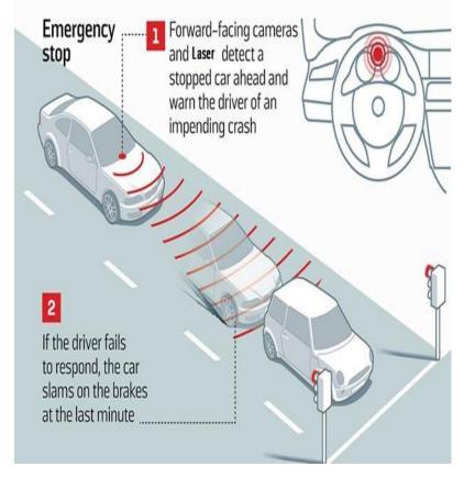
Autonomous emergency braking system is generally designed to activate at highway speeds, as long as the forward collision warning sensors are able to detect the vehicle forward. Newer systems work at slower speeds in towns. However, not all autonomous emergency braking features are able to bring your car to a full stop.
