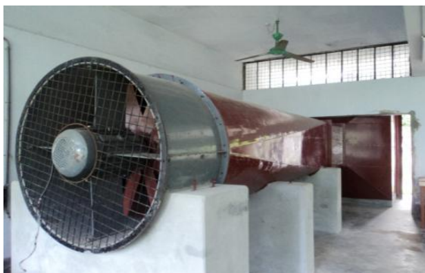
Fig -59: Assembled Wind Tunnel [12]
