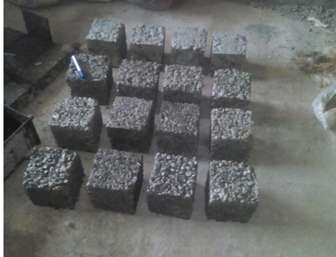
Plate 2: Demolded concrete cubes
