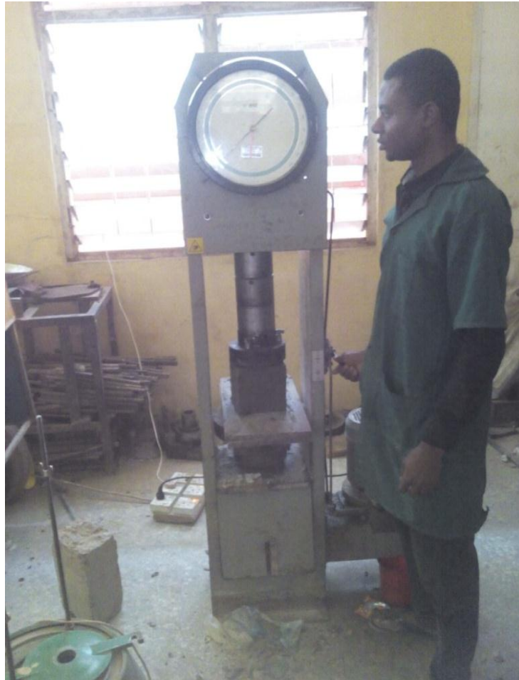
Plate 4: Crushing of Concrete cubes with the U.T.M.
