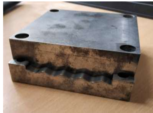
Fig 1 (a): Assembly of upper and lower semi-circular groove corrugated dies
