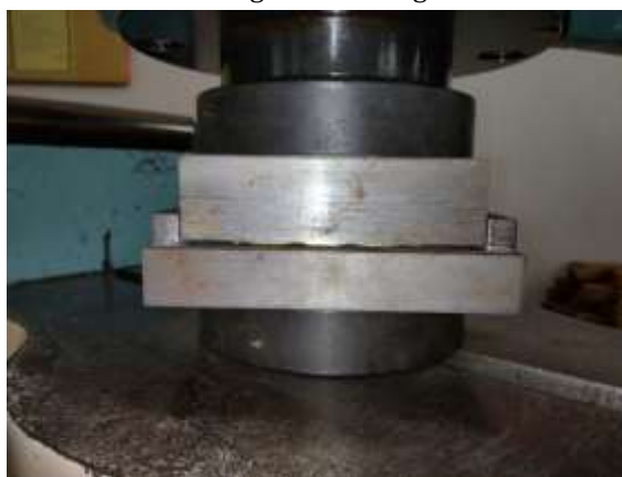
Fig 2 (b): Flattening CGP process using flat dies
