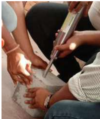
Fig. 3.6: Laboratory procedure For Schmidt hammer test.
