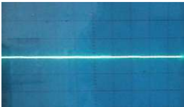
Fig. Waveform of common mode leakage current.
