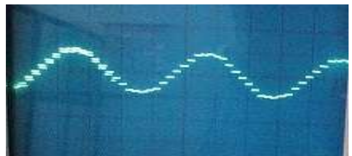
Fig. Waveform of grid current
