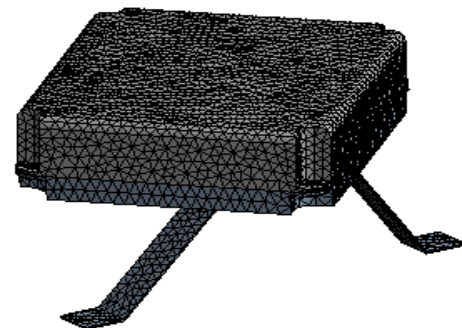
Fig. 4 Meshing of ECU Housing without stiffeners
