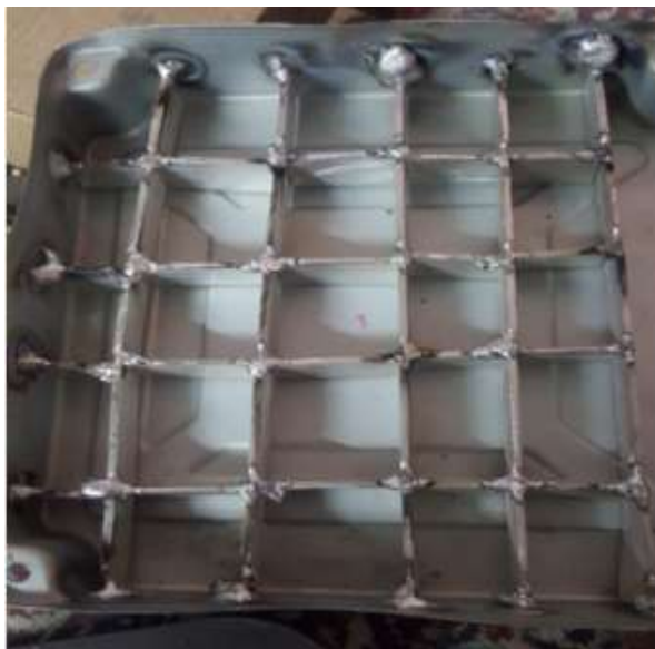
Fig. 15 Model of ECU housing with Stiffener
