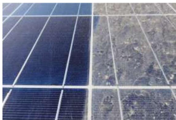
Figure 1: Clean solar panel and dust accumulated solar panel.
