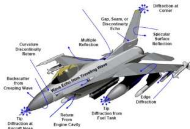
Fig-4: The main surface for radar scattering.
