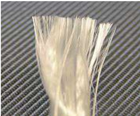
Figure 2. Glass Fibre in Strand Form
