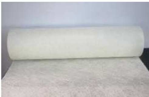
Figure 3. Glass Fibre in Mat Form
