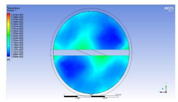
**Fig 4.** Outelt temperature distribution of Twisted tube at 1.2m/s velocity
