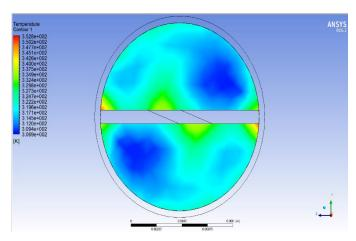
Fig 3. Outlet temperature distribution of Twisted tube at 0.1 m/s velocity
