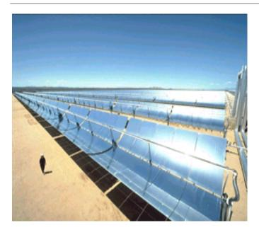
FIG 2.1. Parabolic Trough Collector
