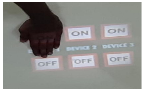
Fig -4: When the device 1 ON option is selected by means of virtual touch, the device starts to work.
