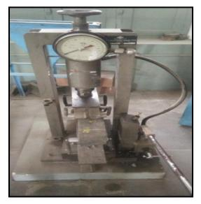
Fig-8: Flexural strength test setup
