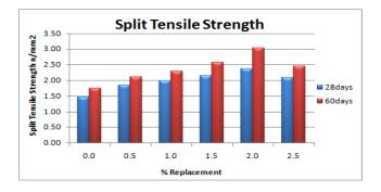
Fig-13: 28 & 60days Split tensile strength (12M)
