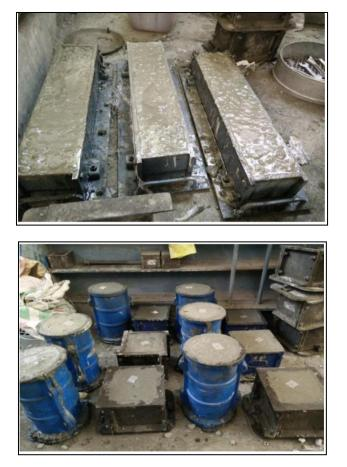
Fig-4: Casting of the concrete specimen
