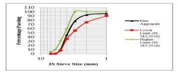
Fig-1: Sieve analysis of Fine aggregate
