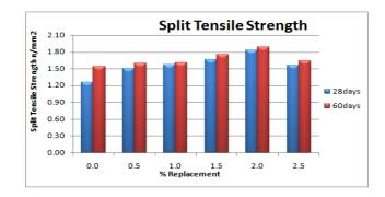
Fig-12: 28 & 60days Split tensile strength (10M)
