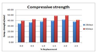
Fig-10: 28 & 60 days compressive strength (12M)
