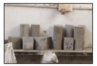
Fig-5: Curing of the concrete specimen
