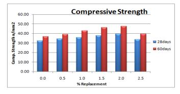
Fig-10: 28 & 60days compressive strength (10M)
