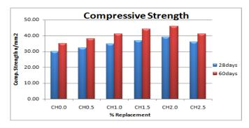
Fig-9: 28 & 60days compressive strength (8M)
