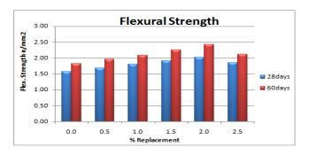
Fig-15: 28 & 60 days Flexural strength (10M)
