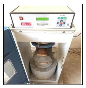
Fig-7: Split tensile strength test setup
