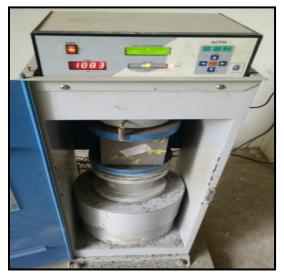
Fig-6: Compressive strength test setup
