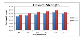
Fig-14: 28 & 60days Flexural strength (8M)
