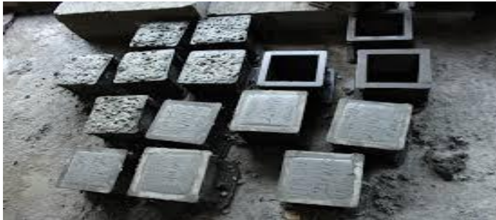
Fig 1. Cube moulds with Concrete
