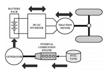
Fig-2: Series hybrid vehicle mechanism
