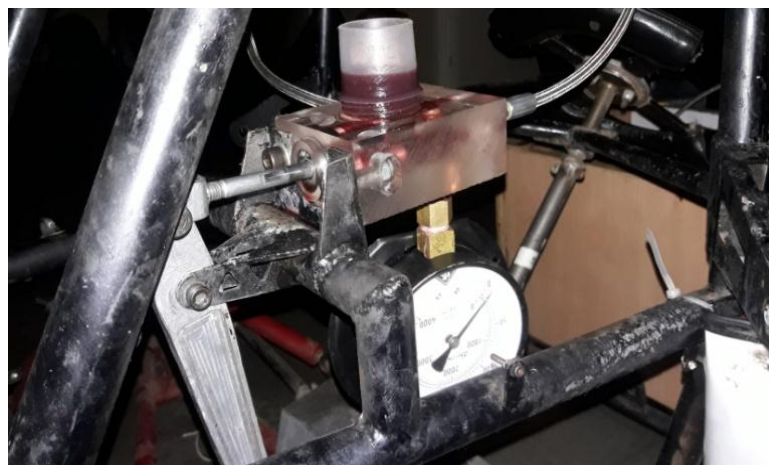
Fig -4: Master cylinder prototype mounted on a chassis with mechanical pressure gauge
