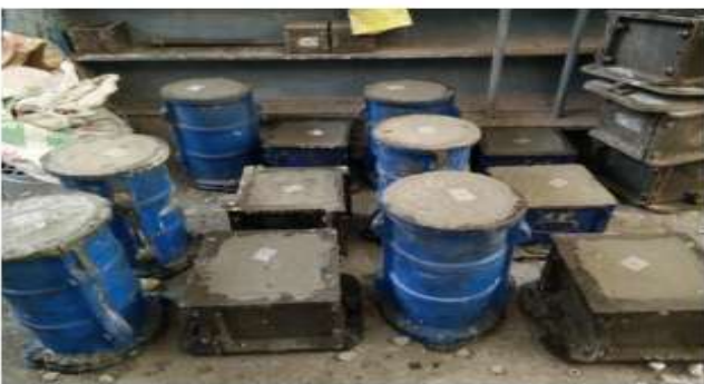
Figure 3: Casting of geopolymer concrete
