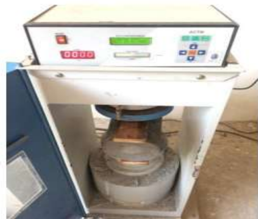
Figure 6: Split tensile testing
