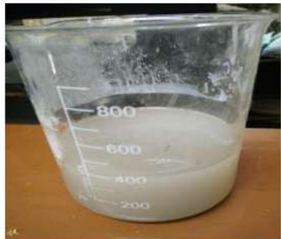
Figure 2: Preparation of alkaline liquid before casting
