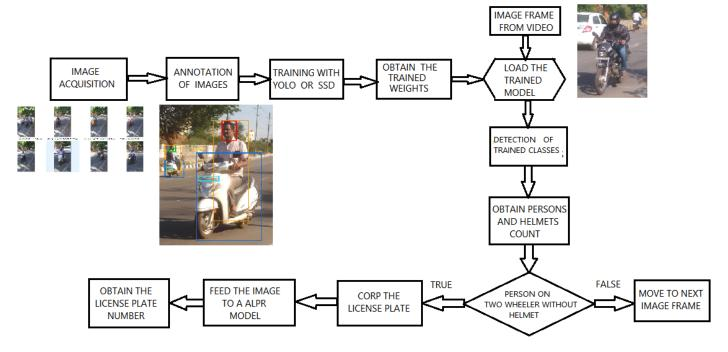
For real-time helmet detection, there is a need for accuracy and speed. Hence a DNN based model You Only Look Once (YOLO) was chosen. YOLO is a state-of-the-art, real-time object detection system.
