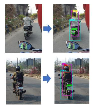
The code extracts the License plate from the Object detector output. The License plate extraction code extracts only from the motor bikes which has a rider who is not wearing helmet and discards the License plate of the motor bikes whose rider has helmet.
