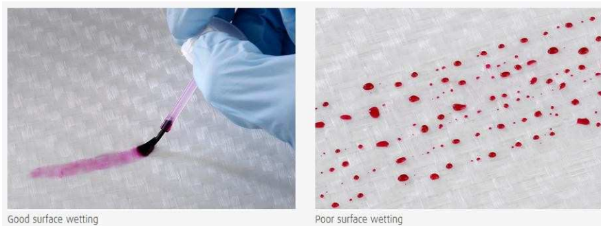
Fig.8: Surface Tension Measurement using Ink Test Pen
