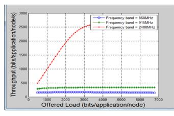
Fig 10: Throughput of different frequency bands
