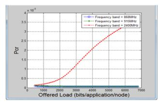
Fig 9: Failure transmission due to retry limits
