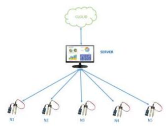
Fig -2: System Architecture
