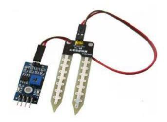
Fig -3: Soil Sensor
