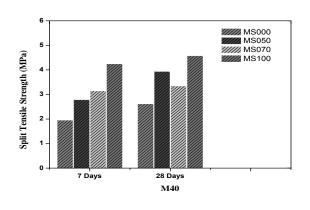
Figure 3.4: Split Tensile strength of cylinder M40
