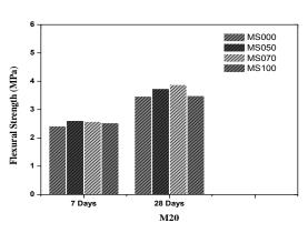
Figure 3.5: Flexural strength of cube M20
