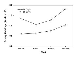
Figure 3.7: Drying Shrinkage of cube M40
