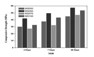
Figure 3.2: Compressive strength of cube M40
