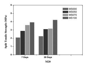
Figure 3.3: Split Tensile Strength of cylinder M20
