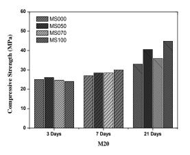
Figure 3.1: Compressive strength of cube M20
