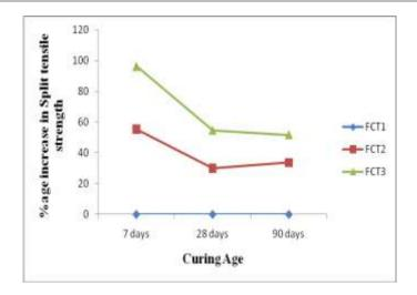
The similar trend was observed at hardened age of 90 days where the results obtained show an increase in split tensile strength of 34% and 52% at W/B ratio of 0.5 and 0.4 in comparison to W/B as 0.6. The decrease in percentage of split tensile strength at 90 days showed that the effect of Silica fume at more curing was less in comparison to that at early ages.
