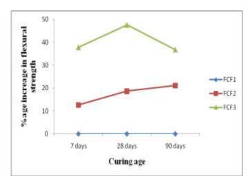
The results obtained at 90 days show an increase in flexural strength of 21% and 37% at water binder ratio of 0.5 and 0.4 in comparison to water binder ratio as 0.6. The decrease in percentage of flexural strength at 90 days has the same reason as discussed earlier.
