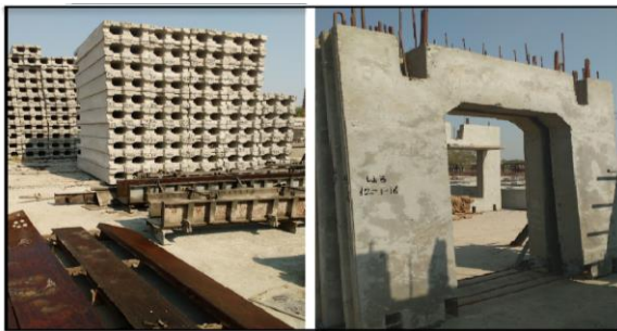
Fig-1: Precast Column Fig-2: Precast Shear Wall
