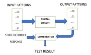
Fig1: Architecture of Test pattern
